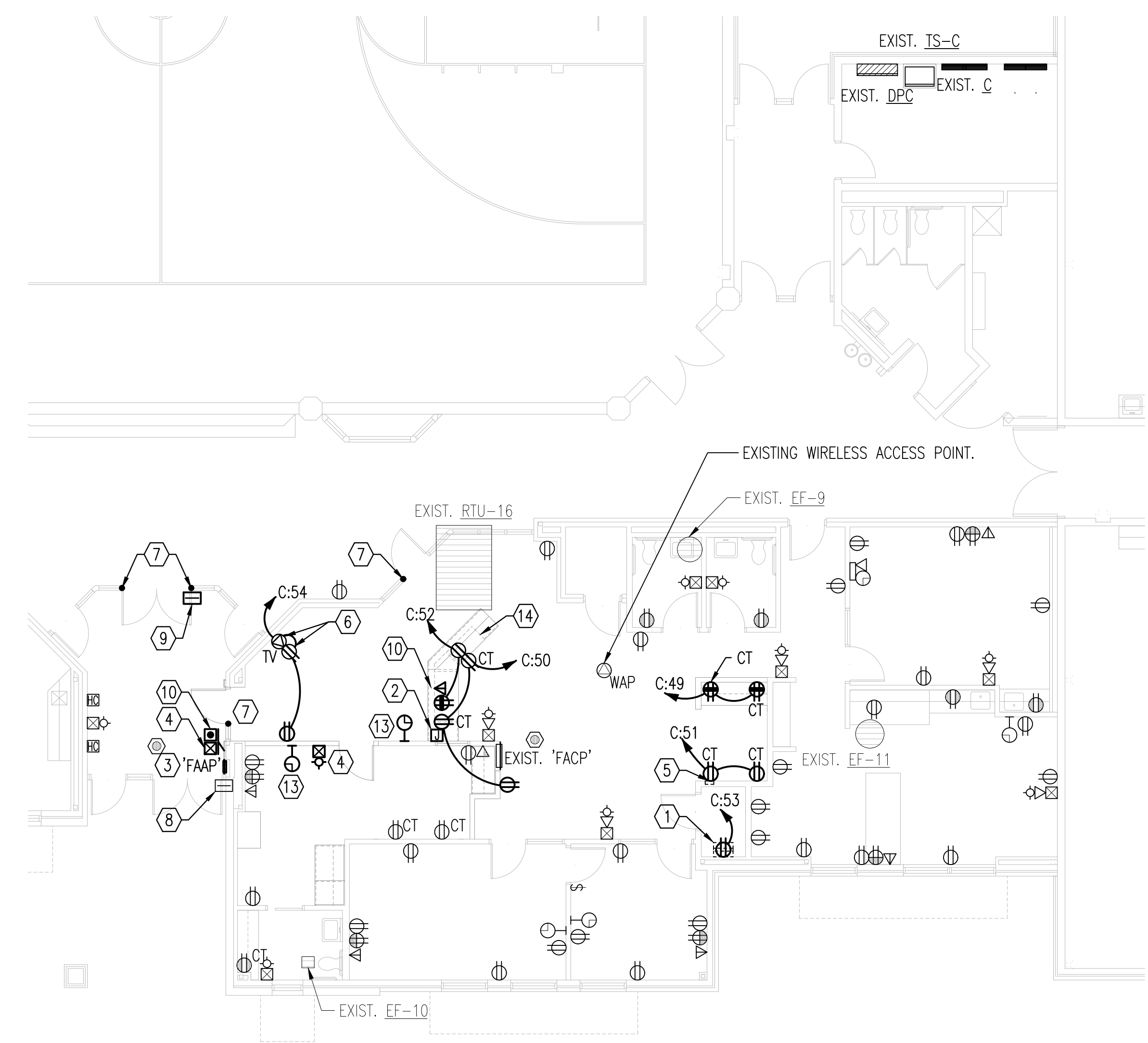
(C) HOLCOMB MIDDLE SCHOOL POWER/LIGHTING PLAN SCALE: 1/8" = 1'-0" N
